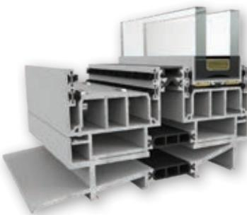
The **MINILINE** is a minimalist sliding glass wall. All aluminium profiles are built into the ground, ceiling and wall. Remains: **only the vertical aluminium profile only 20 mm wide.** Thermally insulated.
